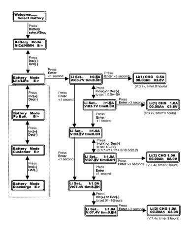
Note: "I" value-----Charge current, 0.5~5.0A provided. "V"value-----Nominal voltage of battery: 1s~6s (means 1 to 6 series pack, voltage is from 3.7v to 22.2v) provied. "tim"value---Max. charging time: default value is 8
