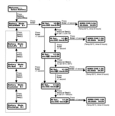
Note: "I" value----Charge current, 0.5~5.0A provided. "ntc" value---Max. temperatuer of battery: 50°C is default value. 45°C ~70°C is provied. "tim" value---Max. charging time: default value is 8 hours. 1 hour to 16 hours provided. 3) Li-Ion/Polymer battery charge operating guide
