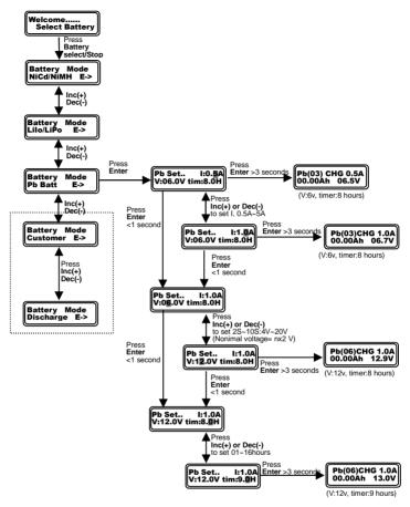
Note: "I" value-----Charge current, 0.5~5.0A provided. "V"value-----Nominal voltage of battery: 2s~10s (means 2 to 10 series pack, voltage is from 4v to 20v) provied. 6V(03S) and 12V(06S) are common. "tim"value---Max. charging time: default value is 8 hours. 1 hour to 16 hours provided. 5) "Customer" special battery setting
