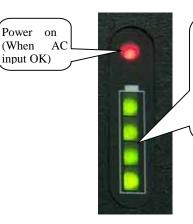
Charging process indicator: Indicate battery capacity from 25% to 100% when charging. All lamps flashing means battery polarity reversed or output shorted. All lamps are "off" means no battery.
